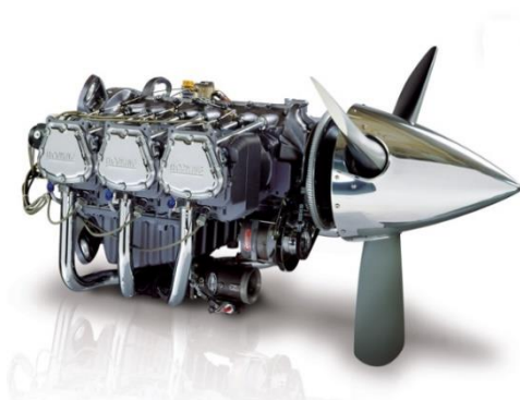
Figure 3. Lycoming IO540K1D5 piston engine model of the Neiva T-25 aircraft. Source: Brazilian Air Force (2023).
