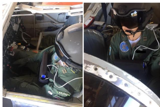
Figure 4. Positioning of the BcMM 2000 equipment inside the T-25 aircraft. Source: Authors.
