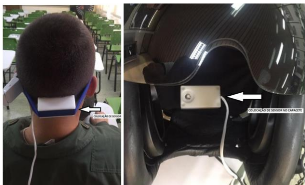
Figure 3. Sensor attached to the pilot's helmet and head. Source: Authors.
